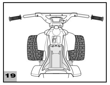
• Fit a hand grip onto each end of the handlebar. If it is difficult to slide the hand grips onto the handlebar, moisten the hand grips with warm water first.
